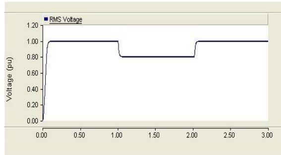
**Fig.2.voltage sag waveform**
